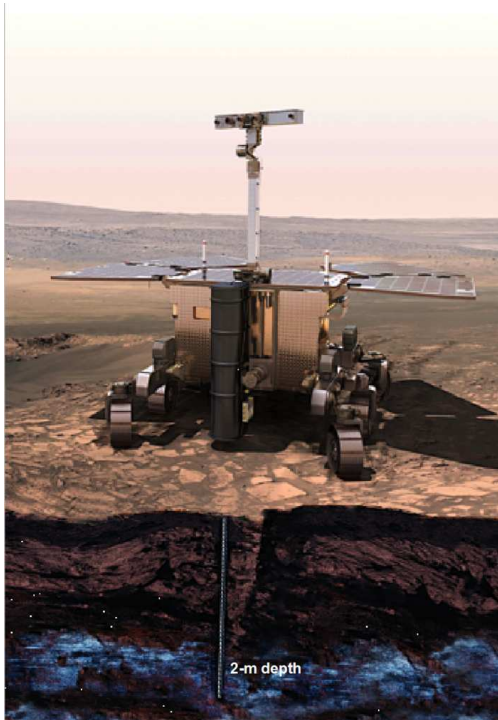
Fig. 1. A picture of the ExoMars Pasteur Rover with the Drilling system: the drill will perform excavations in the Martian subsoil, down to a depth of up to 2 meters
