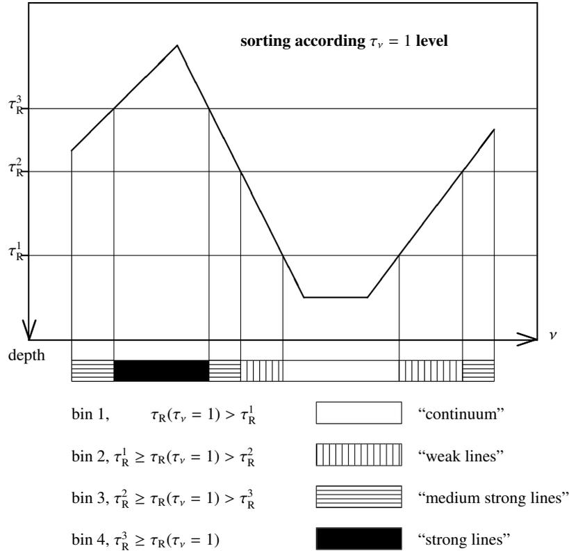
**Fig. 1.** Schematic illustration of the classification of frequency points in the OBM. In the case shown, 4 bins are constructed representing the continuum and increasingly stronger spectral lines. Note, that in general the bins do not form contiguous frequency bands (from Ludwig 1992).
