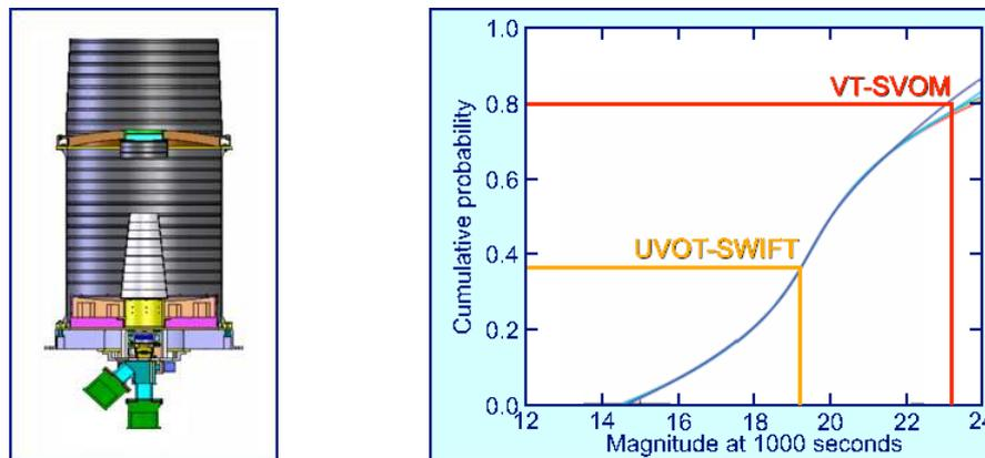
**Fig. 4.** Left: Current VT design. Right: Intrinsic cumulative optical afterglow distribution following Akerlof & Swan (2007) compared to the UVOT and VT sensitivities.
