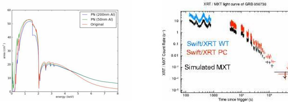
**Fig. 3.** Left: Expected MXT effective area using the pn CCD with different optical filters (blue and green) and using a thinner CCD (red) Right: Simulated MXT light curve of GRB 050730 compared to the XRT data.
