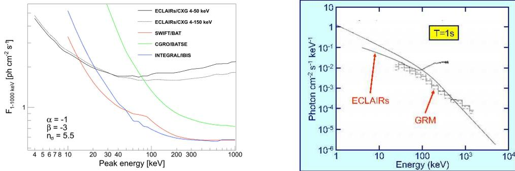
**Fig. 1.** Left: Expected ECLAIRs  $5.5 \sigma$  sensitivity as a function of the peak energy of the GRB (the  $\alpha$  and  $\beta$  parameters of the Band function (Band et al. 1993) are also given), compared to currently flying and past experiments. Right: Combined ECLAIRs-GRM 1 s sensitivity curves compared to an average BATSE GRB spectrum with a 50–300 keV flux of  $1 \text{ photon cm}^{-2} \text{ s}^{-1}$ .
