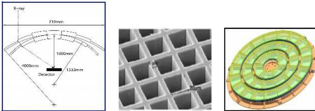
**Fig. 2.** Left: Optical scheme of the MIXS-T/MXT optic. Centre: A close view of the micro-channel plates. Right: assembled MCPs into a complete optic (from Fraser et al. 2009).
