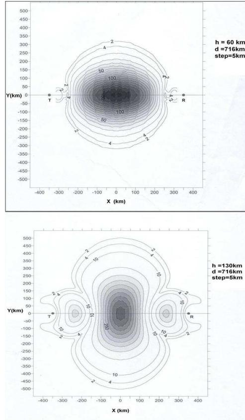
**Fig. 3.** Different gain zones of the BL system at the two height extremes, i.e. for (top)  $h = 60$  km and (bottom)  $h = 130$  km (distance Bologna-Lecce  $d = 716$  km, step = 5 km).
