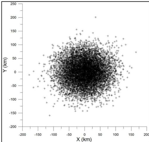
**Fig. 4.** Positions of 3000 echoes on a horizontal plane including the radar baseline, according to the simulation program. Only 30% of the total number was selected with respect to the intensity of the reflected signal. A Gaussian distribution of heights between 55 and 100 km (peaked at 75-80 km) is assumed.
