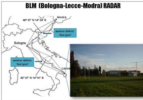
**Fig. 1.** The display of the BLM (Bologna-Lecce-Modra) radar system implemented by a 5-antenna radio-interferometer installed in 2008 at the receiving station in Lecce.
