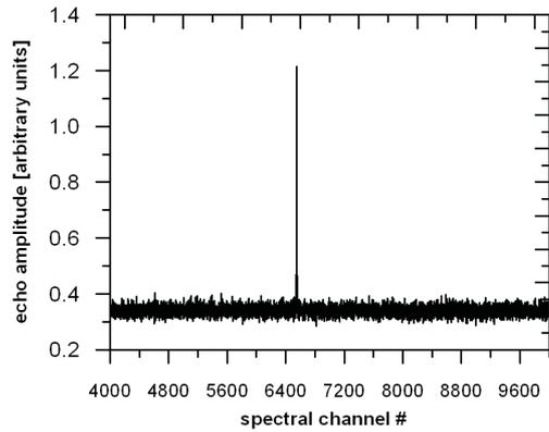
**Fig. 7.** Echo from a not catalogued debris orbiting at a geodetic height of 871.7 km. The echo was detected on April 28, 2009 at 15:26:54.960 UT.
