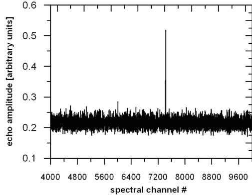
**Fig. 6.** Detection of the small debris 35716 (COSMOS 2251 DEB).
