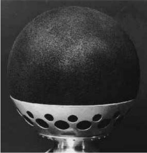
**Fig. 3.** Radar calibrator Tempstat-1. This is an US military target satellite with a 36.0 cm spherical shape launched in LEO polar orbit.
