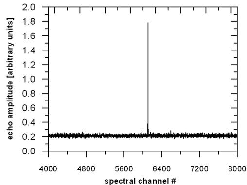
**Fig. 5.** Spectrum of a Fengyun 1C debris radio echo detected by the Medicina RT-32 antenna.
