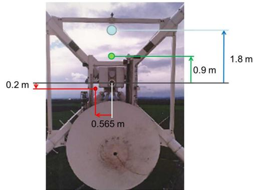
**Fig. 2.** View of the primary focus of the Medicina 32-m radiotelescope. In the figure the positions of the three simulated piggy-back feeds are showed.
