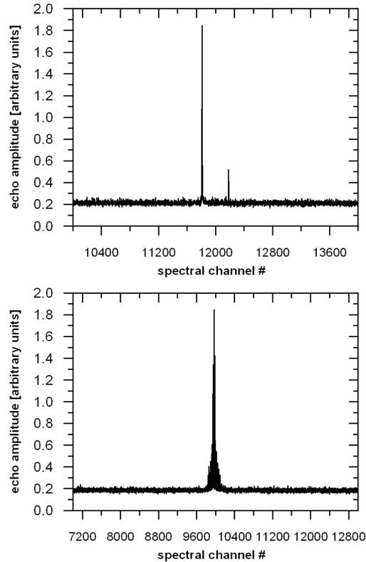
**Fig. 4.** Radar detections of an IRIDIUM 33 (top) and a COSMOS 2251 (bottom) fragments.
