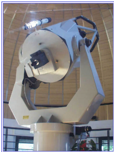
Fig. 1. IRAIT at the Coloti Observatory operated by University of Perugia. This 0.8m telescope was built in collaboration with the Italian Programma Nazionale di Ricerche in Antartide (PNRA), sectors Technology and Earth-Sun Interaction and Astrophysics .
