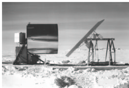
Fig. 1. Telescope at Dome C. The Cassegrain telescope points toward the large flat mirror, which is tilted at 45^{\circ} to steer the beam toward the Zenith.
