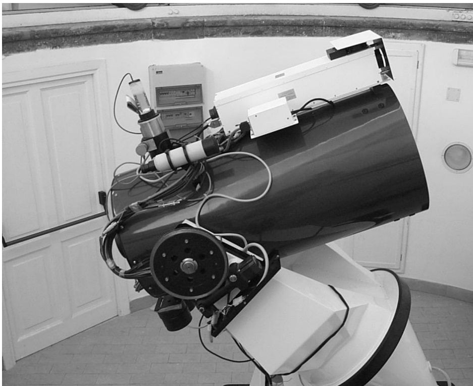
Fig. 1. The 40cm aperture telescope currently in operation in the East tower of the OAC main building is a example of the instrument class that CONCORDIASTRO/Italy plan to install for solar site testing at Dome C.
