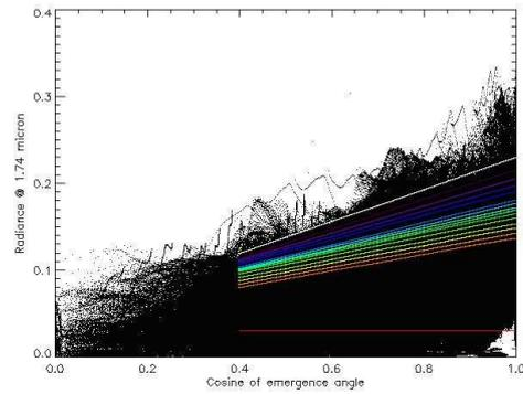
**Fig. 2.** Limb darkening real case: scatter plot of radiance at 1.74  $\mu\text{m}$  as function of cosine of emergence angle. The straight lines are the linear fits used for LD correction. Radiances are in  $\text{W}/\text{m}^2/\text{sr}/\mu\text{m}$ .
