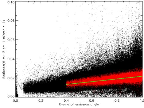
**Fig. 3.** Scatterplot of radiance at  $1.03\mu\text{m}$  as function of cosine of emergence angle. Red points are relative to a same interval of radiance at  $1.74\mu\text{m}$  and surface altitude. These pixels behave in a linear fashion: the green straight line is the best linear fit.
