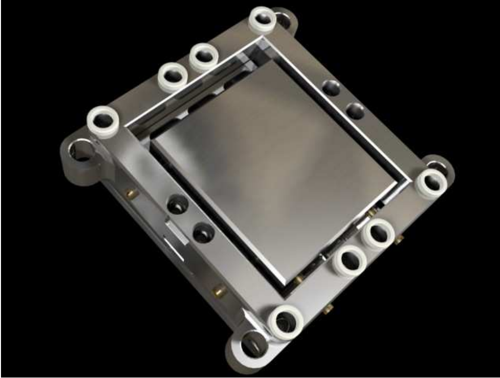
Fig. 3. ISA sensing element. Three of these elements are arranged with the electronics to compose the ISA three-axis accelerometer.
