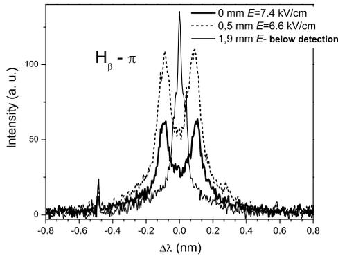
**Fig. 2.**  $\pi$  components of  $H\beta$  line recorded with a polarizer at different distances from the cathode of Grimm type glow discharge. Measured electric field strengths are listed, (Kuraica et al. 2009).
