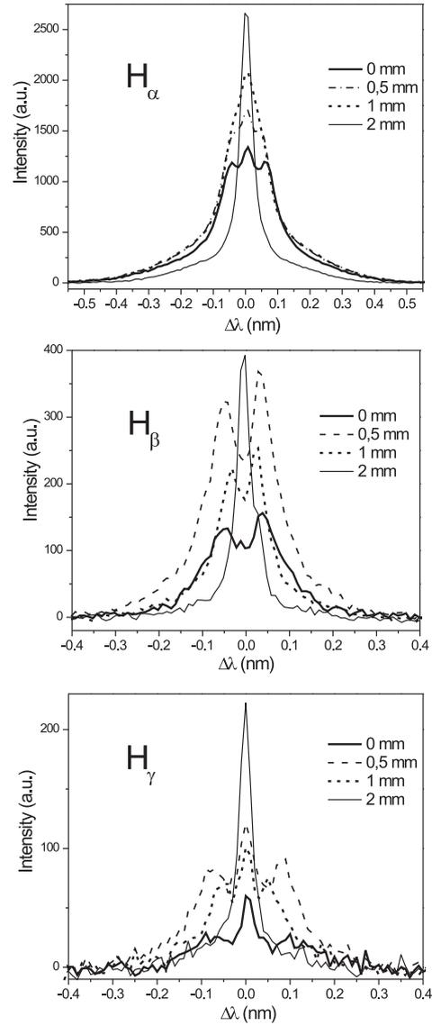
**Fig. 1.** Profiles of hydrogen Balmer series lines recorded at different distances from the cathode of Grimm type glow discharge. Operating conditions: voltage-900 V, pressure-3.8 mbar, (Kuraica et al. 2009).
