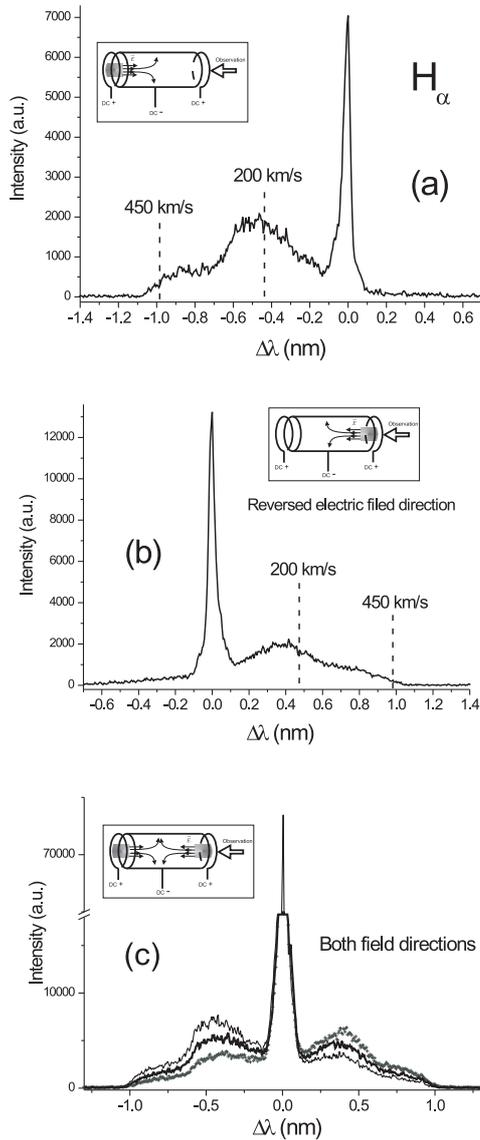
**Fig. 4.** Hydrogen Balmer alpha line with high Doppler shift recorded in hollow cathode discharge: a) Electric field along the line of sight, b) Reversed direction of electric field, c) Electric field present at both directions. Voltage-1.45 kV; pressure-0.4 mbar, (Kuraica et al. 2009).
