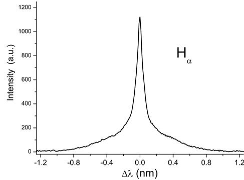
**Fig. 7.**  $H_{\alpha}$  line from electrostatically confined plasma. Voltage-18 kV, pressure-0.8 mbar.
