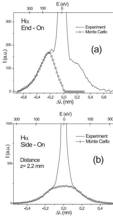
**Fig. 6.** Results of Monte Carlo simulation for obtaining the blue wing of the  $H_{\alpha}$  profile recorded along the E field and far wings of the profile recorded orthogonally to the E field, (Cvetanović et al. 2009).
