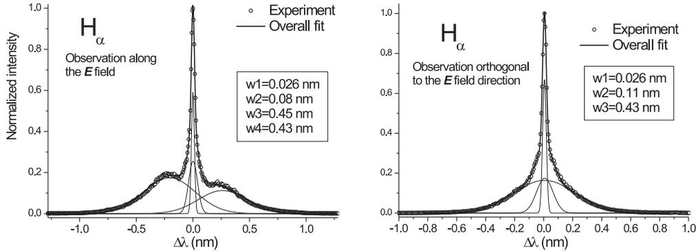
**Fig. 5.**  $H_{\alpha}$  line from Grimm type glow discharge recorded along the direction of electric field (left) and orthogonally to the electric field (right). Voltage-2 kV, pressure-2 mbar.
