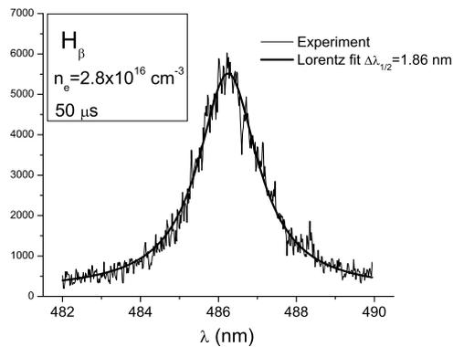
**Fig. 8.**  $H_{\beta}$  recorded at the time of high plasma density of MPC device.
