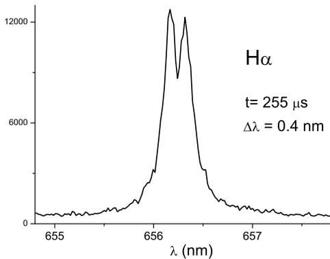
**Fig. 9.** Two-peaked  $H_\alpha$  line recorded long after the termination of MPC discharge, at very low plasma density. Example of inhomogeneous gas absorption.
