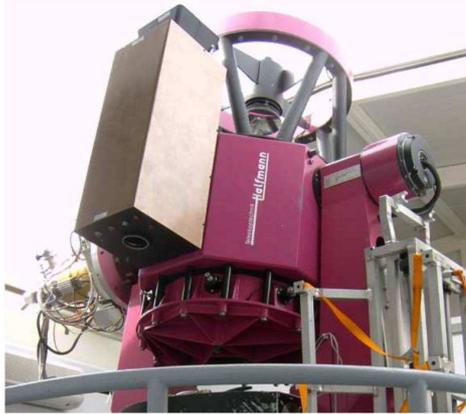
**Fig. 1.** The High-Speed and Wide-Field TORTORA Camera mounted on the top of the 60-cm REM robotic telescope at the European Southern Observatory (ESO) at La-Silla, Chile.
