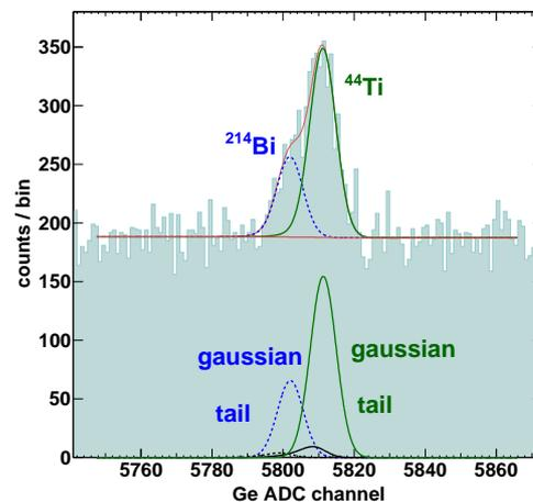
**Figure 2.** Detail of Dergaon spectrum in  $^{44}\text{Ti}$  region in *normal* mode. The fit of  $^{44}\text{Ti}$  and  $^{214}\text{Bi}$  (dotted line) overlapping peaks using a gaussian and a tail is shown.
