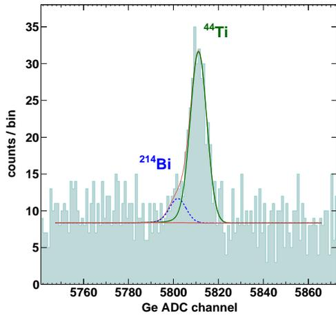
**Figure 3.** Detail of Dergaon spectrum in  $^{44}\text{Ti}$  region in *coincidence* mode, obtained using NaI coincidence window at 1022 keV. As before, the dotted line represents the  $^{214}\text{Bi}$  peak.
