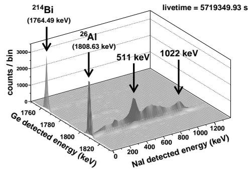
**Figure 1.** Dergaon meteorite Ge-NaI 2-dimensional spectrum in the Ge energy region around  $^{26}\text{Al}$  1808.63 keV peak, for which corresponding NaI detection of  $\beta^+$ -annihilation  $\gamma$ 's is visible. The mostly single- $\gamma$   $^{214}\text{Bi}$  1764.49 keV peak is also shown.
