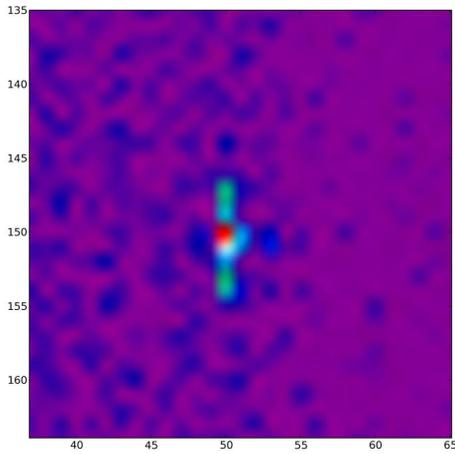
**Fig. 5.** Spectrogram of the echo from debris 8791 recorded by the BEE-2 FPGAs cluster. x-axis: spectral channel; y-axis: time in units of acquired spectra. The intensity of the echo signal is represented in color scale with blue being the lowest and red being the highest intensity.
