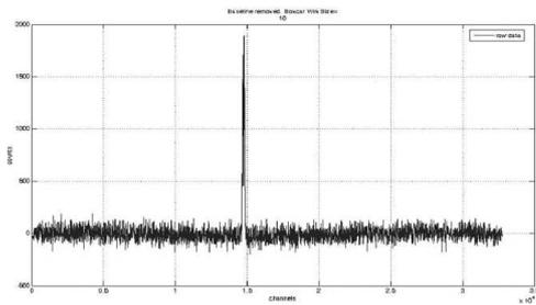
**Fig. 3.** Signal coming from the space debris 29040 as recorded by MSpec0 on July 18<sup>th</sup>, 2007 at 16:32:00 UT
