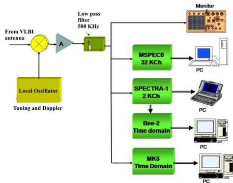
**Fig. 2.** Data acquisition setup scheme with programmable spectrometers, VLBI formatter and high performance BEE-2 FPGAs cluster
