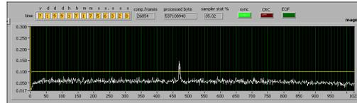
**Fig. 4.** Echo from a not yet catalogued debris orbiting at a geodetic height of 871.7 km detected during the beam parking session. The echo was recorded on July 18<sup>th</sup>, 2007 at 17:17:56 UT.
