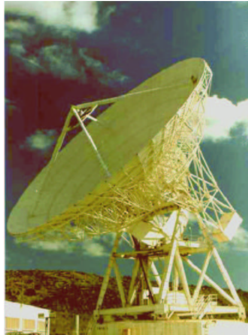
Fig. 2. The Noto 32 meter VLBI dish, equipped with an active mirror ( F_{max} = 43 GHz)
