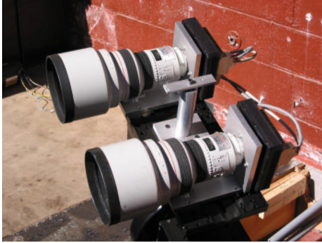
Fig. 1. The XO Mark I system employs twin 200mm Canon EF200 lenses at f/1.8 . This yields a plate scale of 1.058''/\mu\text{m} when coupled with the Apogee Ap8p CCD detectors. Each detector covers 7.2 degrees on the sky and at 25.4''/\text{pixel} .
