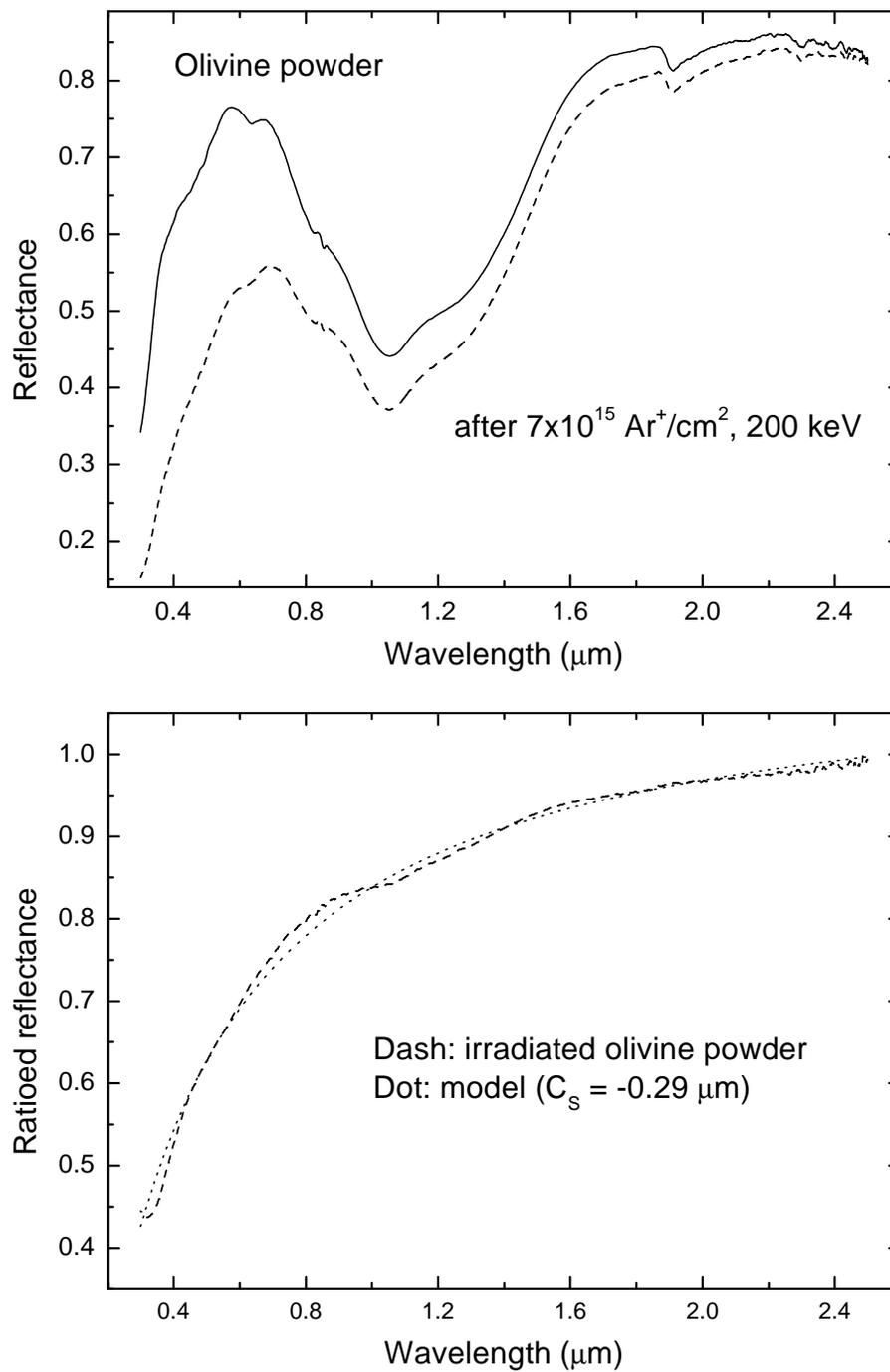
**Fig. 1.** Upper panel: reflectance spectra of powdered San Carlos olivine, before (solid) and after (dashed) ion irradiation. Lower panel: ratio plot of the spectra shown in the upper panel; the dotted curve represents the model obtained using the weathering function  $W(\lambda)$ .
