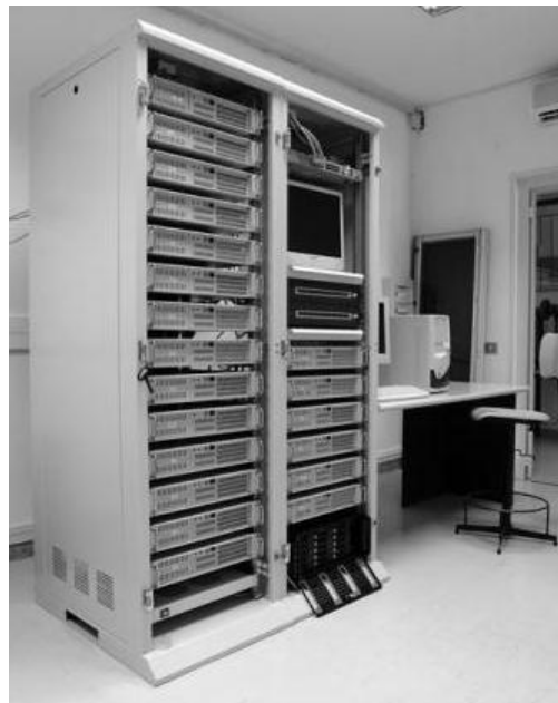
Fig. 4. MANGUSTA, the 20-node Beowulf cluster of the pulsar group.
